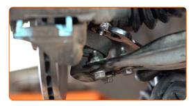
9 Unscrew the front arm fastener. Use a drive socket #16.
