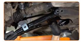
Insert the ball joint into the steering knuckle and fix it with a new nut.
