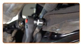
17 Install the rear fastener of the arm.
