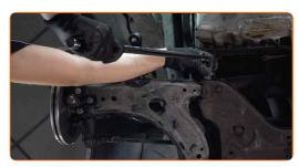
Unscrew the rear arm fastener. Use a drive socket #18.
