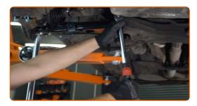
Screw the rear arm fastener. Important! Be sure to use new fasteners. Use a drive socket #18. Use a torque wrench. Tighten it to 70 Nm torque.+90°
