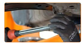
Tighten the ball joint fastening nut. Important! Be sure to use new fasteners. Use a combination spanner #18. Use a torque wrench. Tighten it to 45 nm torque.
