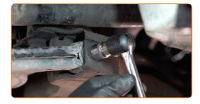
Unscrew the ball joint fastening to the steering knuckle.
