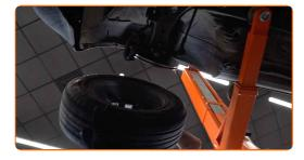
Disconnect the transverse stabilizer fastener from the link. Use a drive socket #16. Use HEX No.H8.
