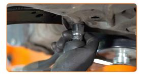
Tighten the ball joint fastening nut. Use a combination spanner #18.
