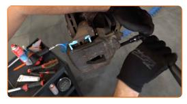
11 Remove the brake caliper.
