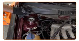
13 Install the upper seal on the firewall.
