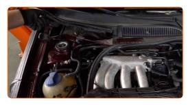
Disconnect the wiring harness from the engine bulkhead and take the wiring out.
