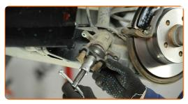
Install the brake caliper and fix it. Use a combination spanner #13. Use a combination spanner #15. Use a torque wrench. Tighten it to 35 Nm torque.
