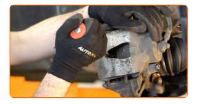
10 Remove the brake caliper.
