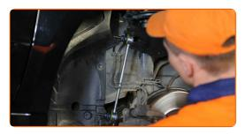
Tighten the fastener connecting the stabilizer link to the shock strut. Use a combination spanner #16. Use Torx T30. Use a torque wrench. Tighten it to 60 Nm torque.
