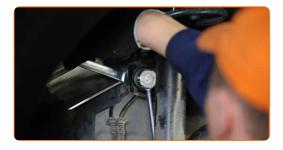
Tighten the fastener connecting the stabilizer link to the stabilizer bar. Use a combination spanner #16. Use Torx T30. Use a torque wrench. Tighten it to 60 Nm torque.
