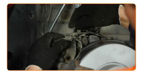
Tighten the fastener connecting the stabilizer link to the stabilizer bar. Use a combination spanner #16. Use HEX No.H6. Use a torque wrench. Tighten it to 60 Nm torque.
