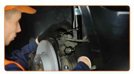
Tighten the lower fasteners connecting the shock strut to the steering knuckle. Use a combination spanner #21. Use a drive socket #21. Use a torque wrench. Tighten it to 120 Nm torque.+90°
