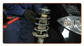
Unscrew the fastener connecting the stabilizer link to the shock strut. Use a combination spanner #16. Use HEX No.H6. Use a ratchet wrench.
