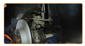
Screw in the fastener that connects the shock strut to the steering knuckle.
