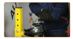
Remove the top strut mount. Use a crowbar.
