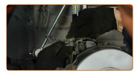
Connect the ABS sensor wiring.
