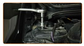
18 Remove the coolant reservoir.
