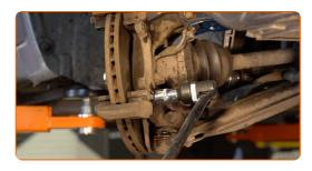
Remove the caliper bracket.
