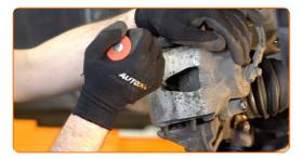
Unscrew the brake caliper fastening. Use a combination spanner #17. Use a drive socket #13. Use a ratchet wrench.
