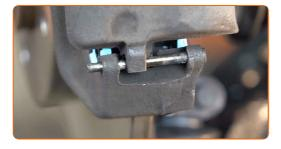
27 Install the brake caliper bracket.
