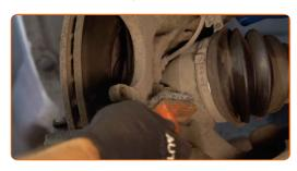
Unscrew the caliper bracket fastening. Use a drive socket #18. Use a ratchet wrench.
