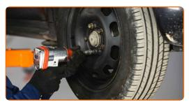
Lower the car and working in a cross order, tighten the wheel bolts. Use wheel impact socket #17. Use a torque wrench. Tighten it to 120 nm torque.
