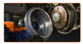
Tigten the brake drum fasteners. Use a flat screwdriver. Use Torx T30. Use a torque wrench. Tighten it to 10 Nm torque.
