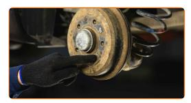
Unscrew the brake drum fastening. Use HEX No.H6. Use a ratchet wrench.
