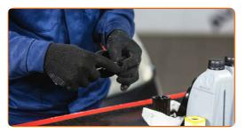
Install new 0-rings (2 pieces) and a new oil filter to their mounting seats on the filter cover. Use a flat screwdriver.
