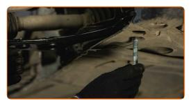
Install the rear fastener of the control arm. Use a hammer.
