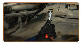
11 Remove the front fastener of the control arm.
