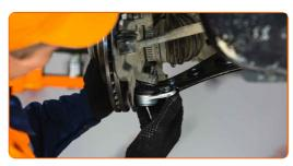
Tighten the ball joint fastener. Use a combination spanner #19. Use a torque wrench. Tighten it to 30 Nm torque.+120°
