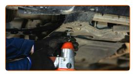
Tighten the rear fastener of the control arm. Use a drive socket #E14. Use a torque wrench. Tighten it to 105 Nm torque.
