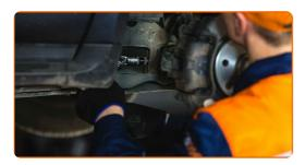
Remove the rear fastener of the control arm. Use a flat screwdriver.
