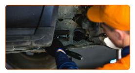
Remove the support from under the arm.
