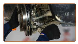
Disconnect the ball joint from the steering knuckle. Use a crowbar. Use a hammer.
