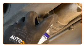
Unscrew the fuel filter bracket fixing bolts. Use a drive socket #8. Use a ratchet wrench.
