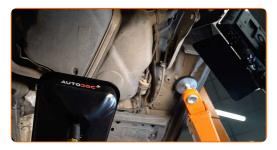
Loosen the fastening clamp of the fuel filter pipe. Use a drive socket #7. Use a ratchet wrench.
