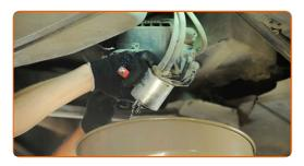
Loosen the fastening clamps of the fuel filter pipes. Use a drive socket #7. Use a ratchet wrench.
