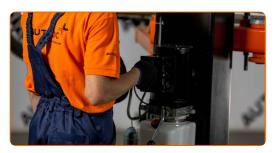
Clean the fuel filter bracket. Use a wire brush. Use WD-40 spray.
