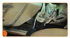
Disconnect the pipe from the fuel filter. Use a flat screwdriver.
