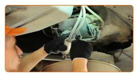
Detach the tubes from the fuel filter. Use a flat screwdriver.
