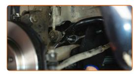
Unscrew the fastener connecting the stabilizer link to the shock strut. Use a combination spanner #17. Use Torx T30. Use a ratchet wrench.
