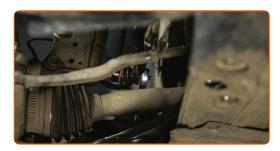
Tighten the fastener connecting the stabilizer link to the shock strut. Use a combination spanner #17. Use Torx T30. Use a torque wrench. Tighten it to 60 Nm torque.
