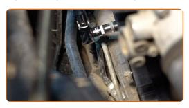
Plug in the ignition coil connector.
