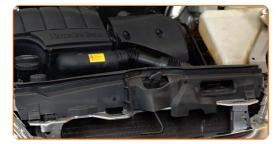
Remove the fender protection cover.
