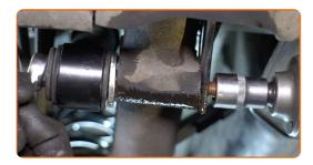
Tighten the lower fastener of the shock absorber. Use a drive socket #18. Use a torque wrench. Tighten it to 80 Nm torque.+90°
