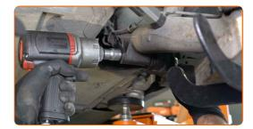
11 Remove the fastening bolt.
