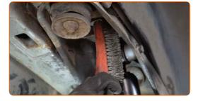
Install the spring on the shock absorber.
