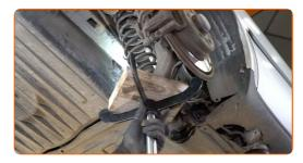
Unscrew the lower fastener of the shock absorber. Use a combination spanner #18. Use a drive socket #18. Use a tap wrench.
