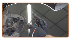
Clean the brake disc fastener. Use a wire brush. Use WD-40 spray.
