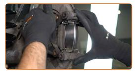
Tighten the brake caliper bracket. Use a drive socket #16. Use a torque wrench. Tighten it to 55 Nm torque.
