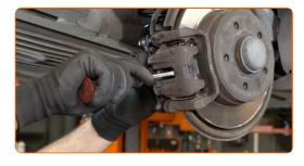
10 Remove the brake caliper.
