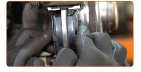
Install the brake caliper and fix it. Use a drive socket #12. Use a torque wrench. Tighten it to 30 Nm torque.
