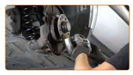
19 Install the brake disc.
