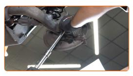
Remove the caliper bracket.
