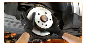
Tighten the brake disc fastening. Use Torx T30. Use a torque wrench. Tighten it to 9 Nm torque.
