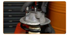
Tighten the shock strut piston rod nut. Use a drive socket #21. Use HEX No.H6. Use a torque wrench. Tighten it to 60 Nm torque.
