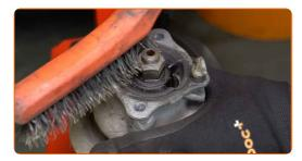
Remove the strut piston rod nut. Use a combination spanner #21. Use HEX No.H6. Use a ratchet wrench.
