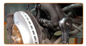
Connect the ABS sensor wiring.
