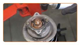
Remove the assembled shock strut.
