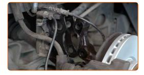
Release the plastic strut mount retainers. Use round-nose pliers. Remove the suspension strut.
