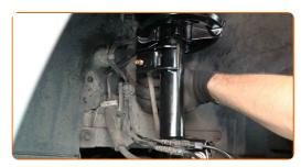
Tighten the fastener connecting the stabilizer link to the shock strut. Use a drive socket #16. Use a torque wrench. Tighten it to 55 Nm torque.
