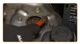
Loosen the upper fasteners of the suspension strut. Use a drive socket #E12. Use a ratchet wrench.
