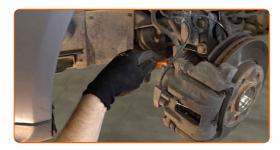
Detach the fastener connecting the ABS sensor cable to the shock strut.
