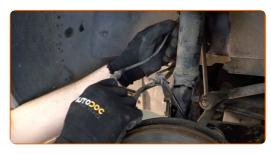
Put a container for gathering brake fluid beneath.
