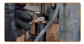
Clean the area where the brake hose is connected to the brake caliper and to the brake circuit pipe. Use a brake cleaner.
