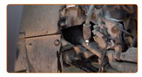
Screw the new brake hose onto the brake caliper.
