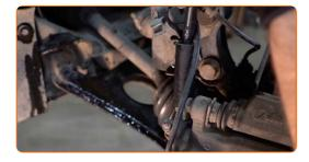
Tighten the fastener connecting the brake pipe to the brake caliper. Use a combination spanner #14. Use a torque wrench. Tighten it to 18 Nm torque.
