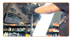
17 Remove the caliper bracket.
