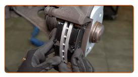
Install the wear sensor on the brake pads.
