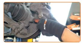
Unscrew the brake caliper fastening. Use a drive socket #12. Use a ratchet wrench.
