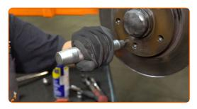
Remove the brake disc.
