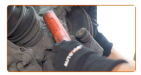
Unscrew the caliper bracket fastening. Use a drive socket #18. Use a tap wrench. Use a ratchet wrench.
