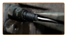
Connect the brake pad wear sensor wire.
