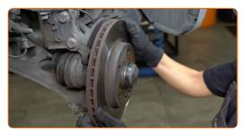
Clean the hub. Use a wire brush. Treat the contacting surface. Use copper grease.
