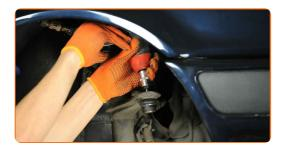
Tighten the tie rod end locknut. Use a combination spanner #14. Use a combination spanner #22. Use a torque wrench. Tighten it to 40 nm torque.
