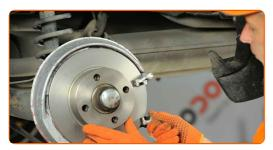
Tighten the brake caliper bracket. Use HEX No.H8. Use a torque wrench. Tighten it to 65 Nm torque.
