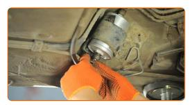
Screw the fastener attaching the fuel supply line to the fuel filter housing. Use a combination spanner #19. Use a combination spanner #22.
