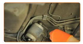
Disconnect the pipe from the fuel filter.
