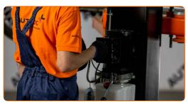
Unscrew the fastener attaching the fuel supply line to the fuel filter housing. Use a combination spanner #19. Use a combination spanner #22.
