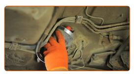
Screw the fixing bolts of the fuel filter bracket. Use a drive socket #10. Use a ratchet wrench.
