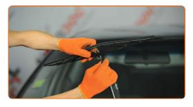
Remove the blade from the wiper arm.
