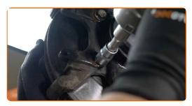
Remove the caliper bracket.
