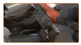
19 Install the brake caliper bracket.
