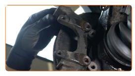
15 Remove the brake disc.
