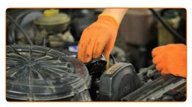
Tighten the oil filler cap.
