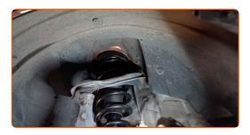
33 Screw the top fastening of the shock strut mount. Do not tighten it.
