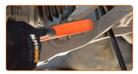
Unscrew the fastening bolt that connects the shock absorber fork with the lower control arm. Use a combination spanner #17. Use a drive socket #17. Use a tap wrench.
