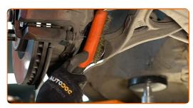
Attach the shock absorber fork to the shock strut.
