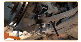
Detach the shock absorber fork from the shock strut. Use a flat metal-working chisel. Use a hammer.
