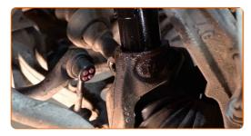
Install the fastening bolt. Use a rubber mallet.
