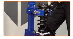
Remove the assembled shock strut. 31
