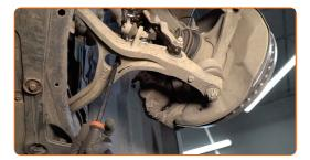
Pull aside the shock strut from its mounting seat.
