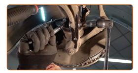
Remove the fastening bolt. Use a pin punch. Use a rubber mallet.
