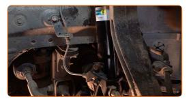
Remove the support from under the arm.
