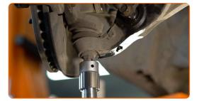
Tighten the fastening bolt that connects the shock strut with the shock absorber fork. Use a drive socket #14. Use a torque wrench. Tighten it to 49 Nm torque.
