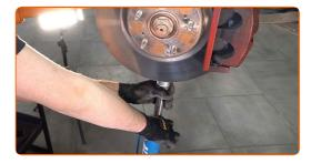
Disconnect the brake hose mounting bracket. Use a drive socket #12. Use a ratchet wrench.
