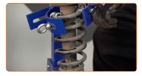
Remove the strut piston rod nut. Use a combination spanner #14. Use HEX No.H6. Use a ratchet wrench.
