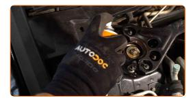
Lower the car and working in a cross order, tighten the wheel bolts. Use a torque wrench. Tighten it to 108 Nm torque.
