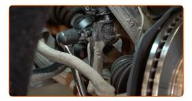
Undo the fastener that connects the shock strut with the shock absorber fork. Use a crowbar. Use a hammer.
