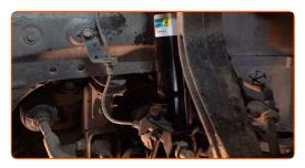
Remove the support from under the arm.
