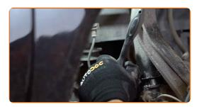
Unscrew the fastening bolt that connects the shock strut with the shock absorber fork. Use a drive socket #14. Use a tap wrench.
