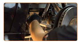
Tighten the fastening bolt that connects the shock absorber fork to the lower control arm. Use a combination spanner #17. Use a drive socket #17. Use a torque wrench. Tighten it to 64 Nm torque.
