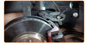
Remove the suspension strut.
