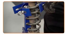
Remove the strut piston rod nut. Use a combination spanner #14. Use HEX No.H6. Use a ratchet wrench.
