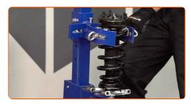
Remove the assembled shock strut.
