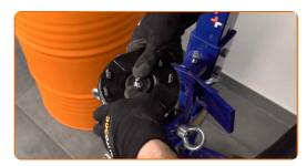
Tighten the shock strut piston rod nut. Use a combination spanner #17. Use HEX No.H6. Use a torque wrench. Tighten it to 29 Nm torque.
