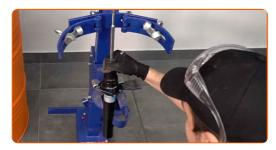
Install the dust sleeve and the bump stop on the new shock absorber.
