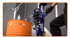
Treat the fasteners of the shock strut mount. Use WD-40 spray.
