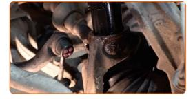
Install the fastening bolt. Use a rubber mallet.
