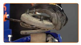
Release the coil spring.
