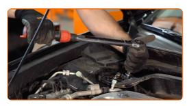
Treat the fasteners of the shock strut mount. Use copper grease.
