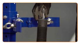
Install the spring on the shock absorber.
