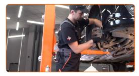
10 Remove the brake caliper.
