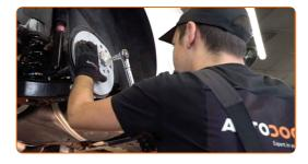
25 Install the brake caliper bracket.
