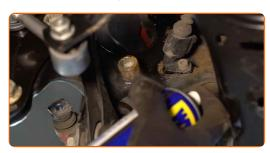
Unscrew the caliper bracket fastening. Use XZN #12. Use a tap wrench. Use a ratchet wrench.
