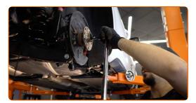
Remove the hub and the bearing together, since they are a sealed unit.
