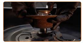
Clean the guiding part of the stub axle. Use WD-40 spray.
