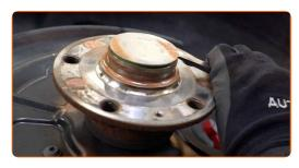
Unscrew the wheel hub axle nut. Use XZN #18. Use a tap wrench.
