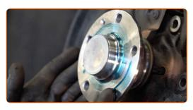
23 Install the brake disc.
