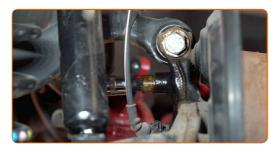
12 Remove the caliper bracket.
