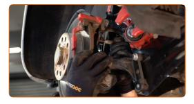
Unscrew the brake disc fastening. Use Torx T30. Use a ratchet wrench.
