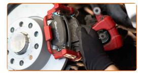
Install the brake caliper and fix it. Use a combination spanner #13. Use a combination spanner #19. Use a drive socket #13. Use a torque wrench. Tighten it to 35 Nm torque.
