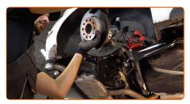
Remove the hub bearing protection cap. Use a crowbar. Use a rubber mallet.
