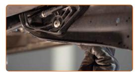
Undo the bracket attaching the parking brake cable to the trailing arm.
