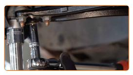
Remove the support from under the arm.
