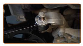
15 Attach the ball joint to the control arm.
