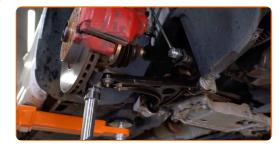
Screw the front arm fastener. Use a drive socket #18. Use a torque wrench. Tighten it to 70 Nm torque.+180°
