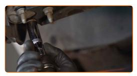
Unscrew the rear fastener connecting the control arm to the subframe. Use a drive socket #15. Use a tap wrench.
