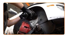
Secure the upper fasteners of the shock strut. Do not tighten it.  $\label{eq:continuous}$
