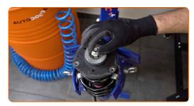
Tighten the shock strut piston rod nut. Use a drive socket #21. Use HEX No.H6. Use a torque wrench. Tighten it to 60 Nm torque.
