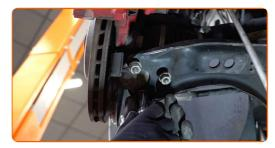
Secure the stabilizer link on the suspension strut. Use a combination spanner #16. Use XZN #6. Use a torque wrench. Tighten it to 65 Nm torque.
