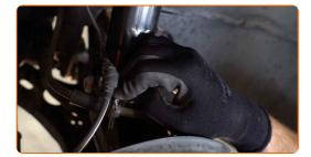
Clean the wheel rim mounting seat. Use a wire brush. Treat the contacting surface. Use copper grease.
