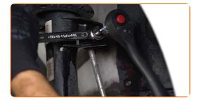
Unscrew the fastener connecting the drive shaft to the wheel hub. Use drive 12-point socket #24.
