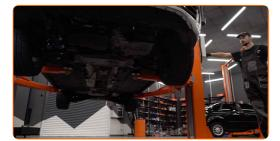
Tighten the shock strut top mount. Use a drive socket #13. Use a torque wrench. Tighten it to 15 Nm torque.+90°
