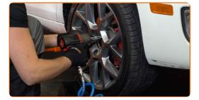
Loosen the wheel hub bolt. Use drive 12-point socket #24. Use a tap wrench.
