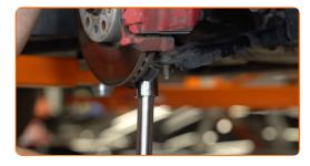
Disconnect the spherical joint from the arm. Use a crowbar.
