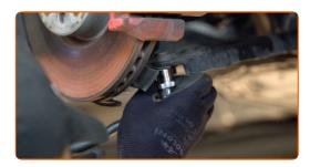
20 Prop up the steering knuckle. Use a hydraulic transmission jack.
