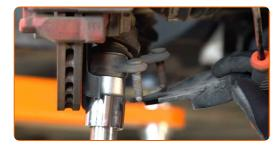
Unscrew the lower fastener connecting the shock strut to the steering knuckle. Use a drive socket #18. Use a combination spanner #18. Use a tap wrench.
