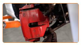
19 Install the brake caliper retaining spring.
