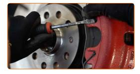
11 Remove the brake caliper.
