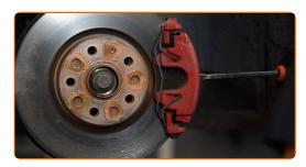
Unscrew the caliper bracket fastening. Use a drive socket #21. Use a tap wrench. Use a ratchet wrench.
