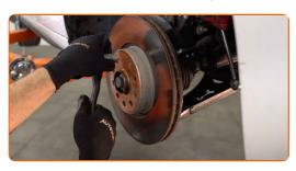
11 Remove the brake disc.
