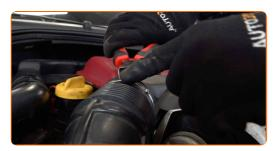
Fasten the clamp on the crankcase ventilation hose. Use combination pliers.
