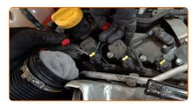
Detach the crankcase ventilation hose clamp from the distribution valve. Use a flat screwdriver. Remove the crankcase ventilation hose.
