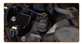
Unscrew the fastener of the chassis (ground) terminal of the ignition coils. Use a drive socket #10.
