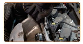
Release the plastic fasteners of the ignition coil connectors. Use flat screwdrivers (2 pieces).
