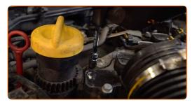
Screw in the fasteners of the crankcase ventilation hose. Use a drive socket #13.
