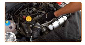
Raise a little the wiring of the ignition coils and move it aside.
