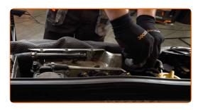
Install the engine cover and secure it.
