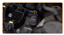
Tighten the chassis (ground) terminal of the ignition coils. Use a drive socket #10.
