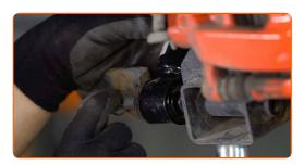
Tighten the lower fastener of the shock absorber. Use a drive socket #19. Use a torque wrench. Tighten it to 85 Nm torque.
