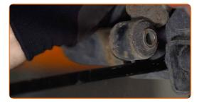
10 Remove the support from under the rear arm.
