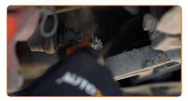
Unscrew the fasteners connecting the stabiliser link to the stabiliser bar. Use box wrench #18. Use HEX No.H5.
