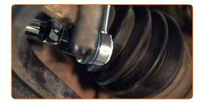
Use box wrench #18. Use a drive socket #18. Use HEX No.H5. Use a torque wrench. Tighten it to 55 Nm torque.
