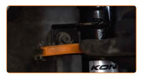
Unscrew the nut and remove the stabilizer rod from the shock strut. Use box wrench #18. Use a drive socket #18. Use HEX No.H5.
