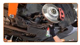
14.1 Install a new rod, tighten the fasteners.
