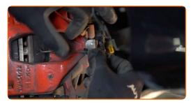
Unscrew the brake caliper fastening. Use a drive socket #13. Use a ratchet wrench.
