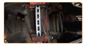
Clean the brake pad clips. Use a wire brush. Use a brake cleaner.
