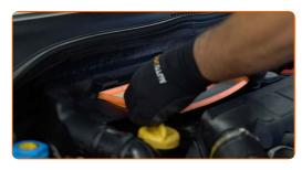
Cover the intake manifold passages with a microfibre towel to prevent dust and dirt from getting inside.
