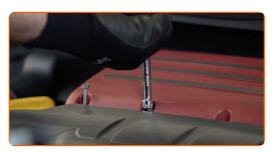
11 Remove the fender protection cover.
