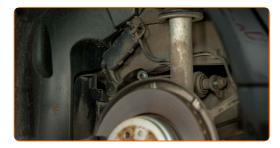
Unscrew the fastener connecting the control arm to the rear knuckle. Use a combination spanner #21. Use a drive socket #10. Use a ratchet wrench.
