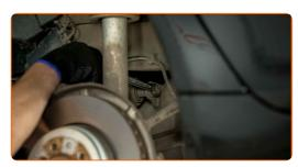
Remove the front fastener of the control arm. Use a crowbar. Use a flat screwdriver.
