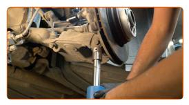
Tighten the fastener connecting the suspension arm to the rear knuckle. Use a drive socket #21. Use a torque wrench. Tighten it to 165 Nm torque.
