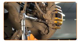
Connect the brake pads wear sensor.
