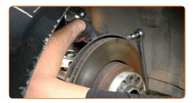
Tighten the arm fastening to the subframe. Use a combination spanner #18. Use a drive socket #18. Use a torque wrench. Tighten it to 100 Nm torque.
