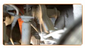
Unscrew the arm fastening from the subframe. Use a combination spanner #18 (2 pieces).
