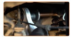
Screw in the fastener that connects the control arm to the rear knuckle. Use a drive socket #21. Use a ratchet wrench.
