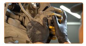
Tighten the brake caliper bracket. Use a drive socket #18. Use a torque wrench. Tighten it to 110 Nm torque.
