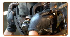
Screw on the fastening nut that connects the tie rod end to the steering knuckle. Use a drive socket #21. Use a ratchet wrench.
