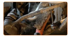
Loosen the lock nut securing the tie rod end to the tie rod. Use a combination spanner #24.
