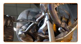
Tighten the fastening nut connecting the tie rod end to the steering knuckle. Use a drive socket #21. Use a torque wrench. Tighten it to 165 nm torque.
