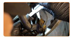
Unscrew the end fastening nut to the steering knuckle. Use a drive socket #21. Use a ratchet wrench.
