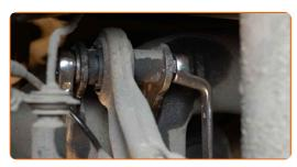
Clean the shock strut fasteners. Use a wire brush. Use WD-40 spray.
