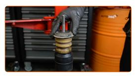
Install the spring on the shock absorber.
