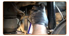
Attach the rear knuckle to the suspension control arm.
