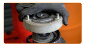
Release the coil spring.
