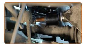
Screw in the lower fastener of the shock strut. Use a combination spanner #18.
