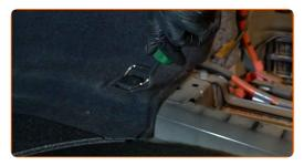
Unscrew the fasteners of the boot front side lining. Use Torx T40. Use a ratchet wrench.
