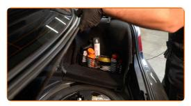
Remove the plastic clip of the boot front side lining. Use a clip removal tool.
