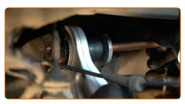
Screw in the fastener that connects the control arm to the rear knuckle. Use a drive socket #21. Use a ratchet wrench.
