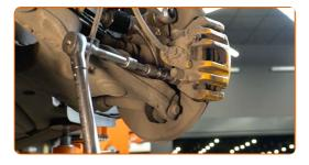
62 Connect the brake pads wear sensor.
