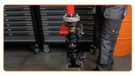
Remove the assembled shock strut.
