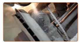
Unscrew the fastener connecting the control arm to the rear knuckle. Use a combination spanner #21. Use Torx T40. Use a ratchet wrench.
