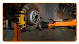
Disconnect the brake pads wear sensor.
