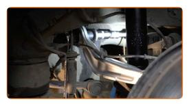
Tighten the lower fastening of the shock absorber. Use a drive socket #18. Use a torque wrench. Tighten it to 100 Nm torque.
