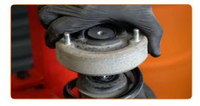
Release the coil spring.
