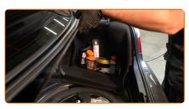
Remove the plastic clip of the boot front side lining. Use a clip removal tool.
