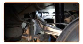
Tighten the lower fastening of the shock absorber. Use a drive socket #18. Use a torque wrench. Tighten it to 100 Nm torque.
