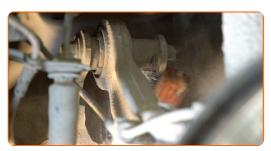
Unscrew the arm fastening from the subframe. Use a combination spanner #18 (2 pieces).
