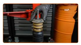
Install the spring on the shock absorber.
