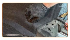
Screw the fasteners of the boot front side lining. Use Torx T40. Use a ratchet wrench.
