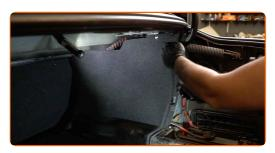
75 Install the plastic clip of the boot front side lining.
