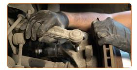
27 Unscrew the top fastening of the shock strut mount.
