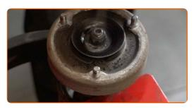
Remove the strut piston rod nut. Use HEX No.H6. Use a drive socket #18. Use a ratchet wrench.
