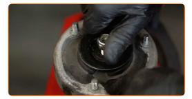
Tighten the shock strut piston rod nut. Use HEX No.H6. Use a drive socket #18. Use a torque wrench. Tighten it to 27 Nm torque.
