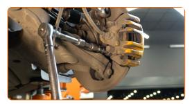
64 Connect the brake pads wear sensor.
