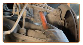
Unscrew the lower fastener of the shock absorber strut. Use a combination spanner #18.
