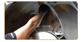
Treat the shock strut rod. Use copper grease.
