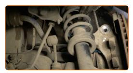
30 Set the shock absorber strut on the spring compressor tool.
