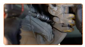
17 Remove the brake caliper together with its bracket.
