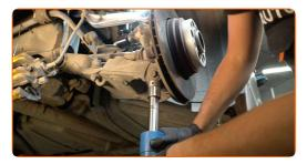
Tighten the fastener connecting the suspension arm to the rear knuckle. Use a drive socket #21. Use a torque wrench. Tighten it to 165 Nm torque.
