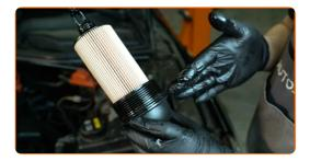
Install a new oil filter housing cover and tighten it. Use a drive socket #32. Use a torque wrench. Tighten it to 25 Nm torque.
