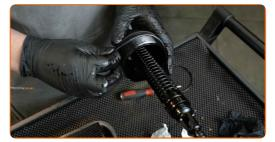
Install the new oil filter to the mounting seat on the filter cover.
