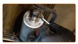
Loosen the fuel filter mounting. Use a drive socket #10. Use a ratchet wrench.
