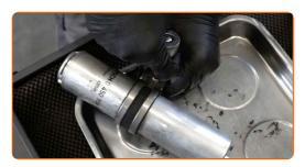
9 Remove the fuel filter fastening bracket.
