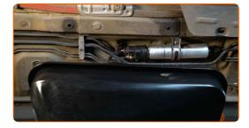
Remove the snap ring of the fuel pressure regulator retainer clip. Use a flat screwdriver.
