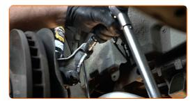
Tighten the fastener connecting the stabilizer link to the stabilizer bar. Use a drive socket #16. Use a torque wrench. Tighten it to 65 Nm torque.
