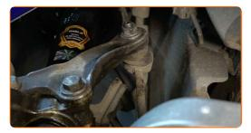
Unscrew the fastener connecting the stabilizer link to the stabilizer bar. Use a drive socket #16. Use a ratchet wrench.
