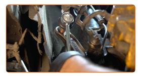
Tighten the stabiliser link fastener. Use a drive socket #16. Use a ratchet wrench.
