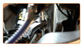
Tighten the fastener connecting the stabilizer link to the shock strut. Use a drive socket #16. Use a torque wrench. Tighten it to 65 Nm torque.
