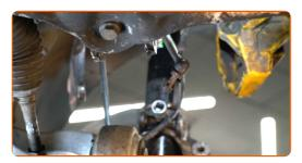
Unscrew the wheel hub axle nut. Use a drive socket #18. Use a ratchet wrench.
