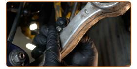
Treat the hub where it contacts the brake disk. Use copper grease.
