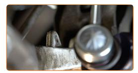
Unscrew the rear fastener connecting the control arm to the subframe. Use a combination spanner #18. Use a drive socket #18. Use a ratchet wrench.
