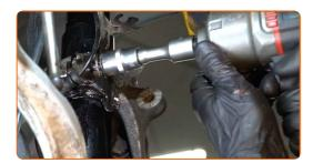
Unscrew the fastener of the stabiliser link bracket. Use a drive socket #16. Use a ratchet wrench.
