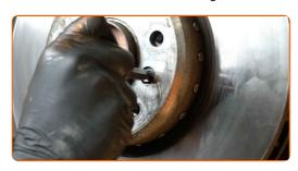
Remove the brake disc.
