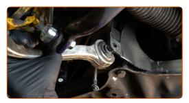
Install the rear fastener of the arm.
