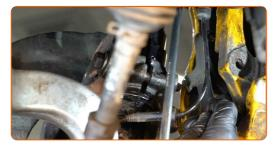
Remove the support from under the steering knuckle.
