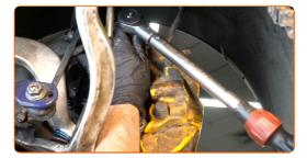
Connect the ABS sensor wiring.
