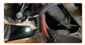
Unscrew the fasteners of the headlight levelling sensor. Use a drive socket #10. Use a ratchet wrench.
