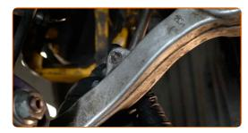
Screw in the fasteners of the headlight levelling sensor. Use a combination spanner #9. Use a drive socket #10. Use a ratchet wrench.
