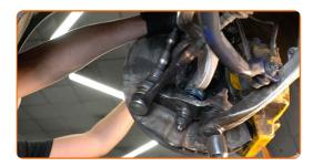
Remove the support from under the arm.
