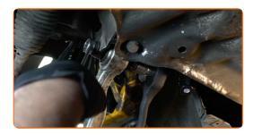
Reconnect the headlight levelling sensor.
