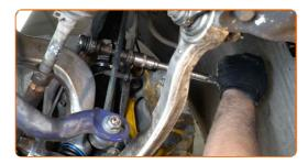
Tighten the fastener of the stabiliser link bracket. Use a drive socket #16. Use a torque wrench. Tighten it to 65 Nm torque.
