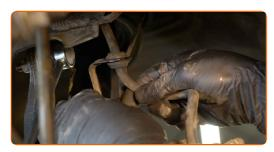
Tighten the lower fasteners connecting the shock strut to the steering knuckle. Use a combination spanner #18. Use a drive socket #18. Use a torque wrench. Tighten it to 81 Nm torque.
