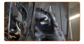
Disconnect the ABS sensor wiring.
