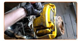
Unscrew the caliper bracket fastening. Use a drive socket #18. Use a tap wrench.
