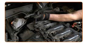
Remove the back section of the engine cover.
