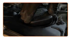
37 Screw in the fastening screws of the air filter cover. Use HEX No.H5. Use a ratchet wrench.
