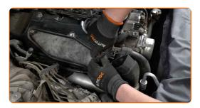
Unscrew the fasteners of the back section of the engine cover. Use HEX No.H5. Use a ratchet wrench.
