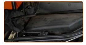
Unscrew the fasteners of the bottom part of the cabin filter housing. Use Torx T25. Use a ratchet wrench.
