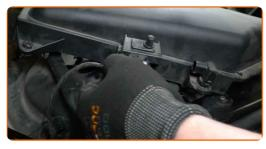
Remove the cabin filter housing seal.
