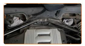
Unscrew the fasteners of the diagonal braces. Use Torx T40. Use a ratchet wrench.
