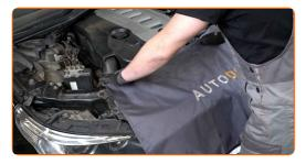
Unscrew the fasteners of the suspension strut mount cover. Use a Phillips screwdriver. Use a clip removal tool.
