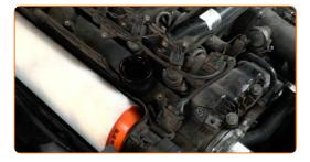
Reinstall the air filter cover. Fasten it.
