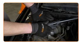
Screw in the fasteners of the suspension strut mount cover. Use a Phillips screwdriver.
