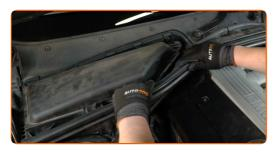
Remove the fender protection cover.
