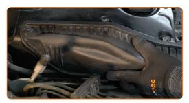
Screw in the fastener of the air intake pipe. Use HEX No.H5. Use a ratchet wrench.
