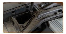
Remove the bottom part of the cabin filter housing.
