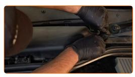
Detach the connectors from the climate control sensors.
