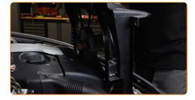
Tighten the cooling fan fastener. Use a combination spanner #32 (2 pieces). Use a torque wrench. Tighten it to 33 Nm torque.
