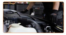
Remove the fan shroud clips. Use a clip removal tool.
