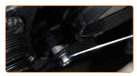
Pull aside the V-ribbed belt tensioner pulley. Use a combination spanner #24.
