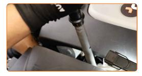
20 Install the fan shroud clips.
